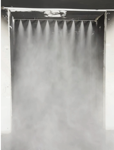
Sinorix high-pressure water mist spray bar creating a protective water mist curtain during fire demonstration
