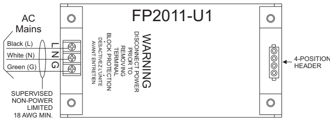
Figure 2 Wiring the FP2011-U1
